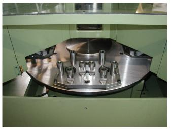
Loading area protected by light beam sensor. Fixture to lay down the workpieces. The workpieces will not be clamped or fixed.
