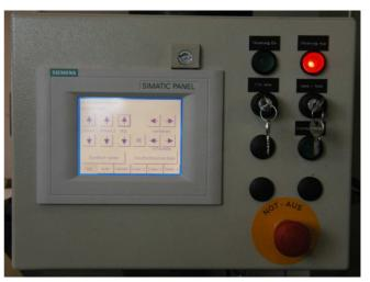
Machine control panel with Siemens touch screen Direct maintenance or modification of parameters is by this easy menu in very short time possible.
