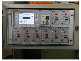
Control box of "Artis" torque control system with visualising of every spindle torque and the possibility to see the torque – time diagram of any spindle. Additionally the spindle which made error can easily be seen. In connection with automatic unloading system the not correct machined workpieces can be taken out of machine. Three following wrong parts will stop the machine.
