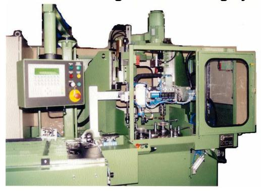
Kind of machining: boring of 4 holes and tapping of 4 tapps M8 into sintered metal type D30 Production capacity: 6 pieces per minute
