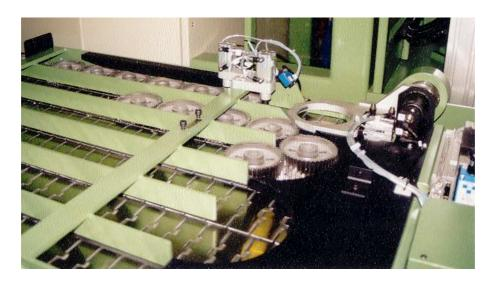
In magazine the workpieces will be singled, pre-orientated and given to swing unit.
