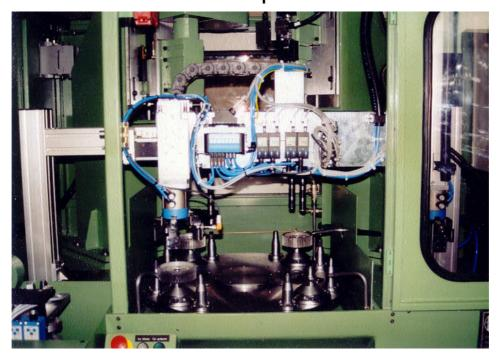
From align system (far left) the workpiece will be loaded to the correct position on the rotary indexing table being set piece recording. By the 90 degrees indexing the workpiece reaches in succession to the boring station in the tapping station and the removal station.
