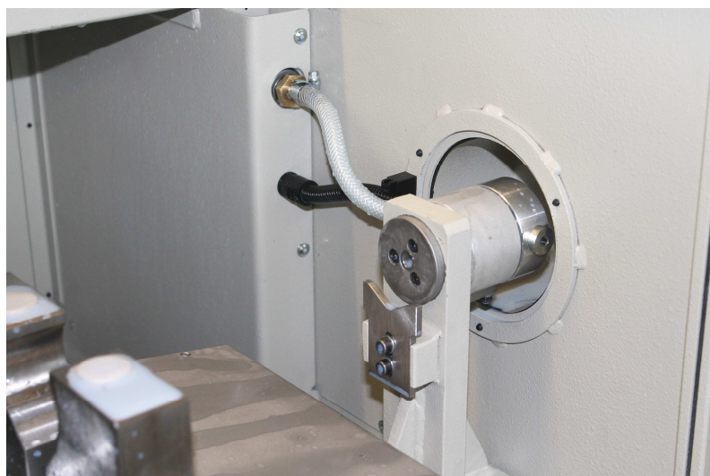
Picture shows: Rear length stop with integrated pre-deposit and coolant inlet (option)
