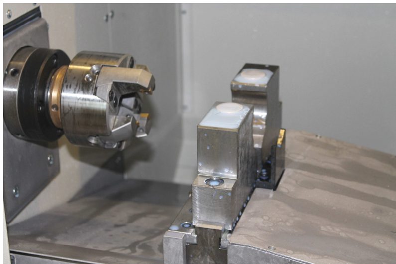
Picture shows: Centering vice in pneumatic design with enclosing jaws and end machining tool
