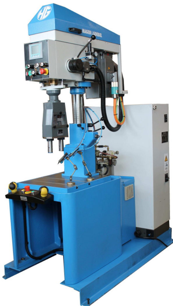
Type HG-22 Servo with motor power 22KW (60% ED) in box base design, multi-spindle head and additional options.
